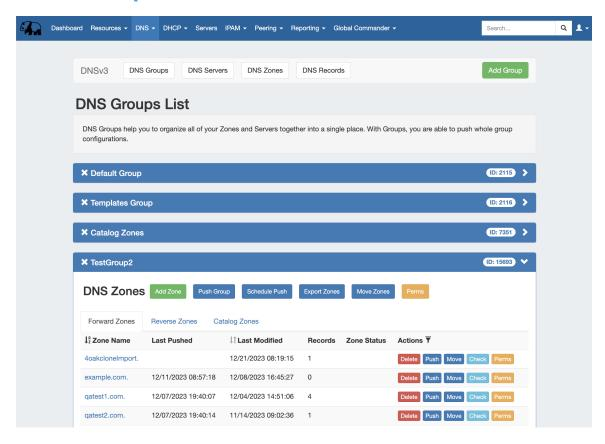
The DNS tab Groups List allows you to create, view, and manage groups of DNS servers and zones. Using groups, you can configure and push selected combinations of zones at one time.
