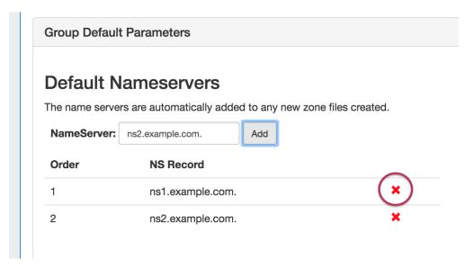
Change the order of multiple Nameservers by left-clicking (holding the mouse button down) over the NS record to move, dragging to its desired placement, then releasing the mouse button.
