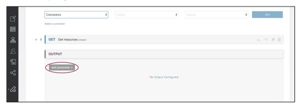
Each Output parameter consists of a number of parts: the parameter name, the parameter type, and the type details. Each parameter requires a distinct name. This is the name used in the return payload.
