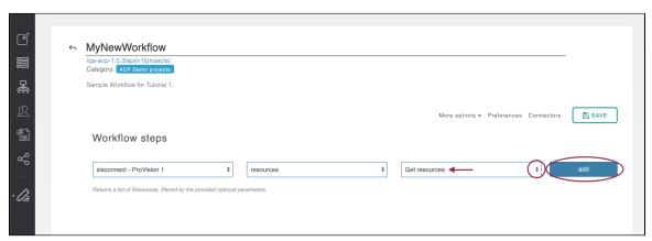
The new step is added to the main ACP work area. An 'Output' step is automatically created below it.
