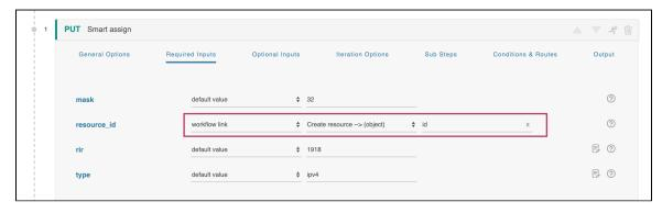
When the 'workflow link' option is selected the form expands to gather the necessary information. The middle drop-down selects what step you will be taking this information from. Once a step is selected, the rightmost 'property' box accepts the name of a parameter.
