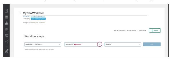
The final box will pull in all of the specific endpoints belonging to that family. Select the specific endpoint action to perform, then click "add" to create the step.
