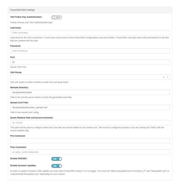
After entering the server-specific settings in this section, you can click the "Test Connection" button at the bottom right of the page to test the server connection and authentication.
